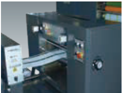
UV上光单元 Flexo vanishing unit
