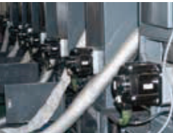
无轴传动 Shaftless driving system
