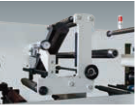
纵切反转贴合 longitudinal cutting and reverse laminating
