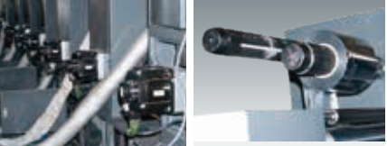
无轴传动 Shaftless driving system 冷烫金 Cold stamping unit
